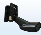
Specially designed for salt water or downrigger tracking with built-in temp sensor, and up to 90° of effective fish detection coverage with 50 kHz – and up to 40° with 200 kHz – using high echosounder sensitivity settings. Not for shoot-thru-hull installation
