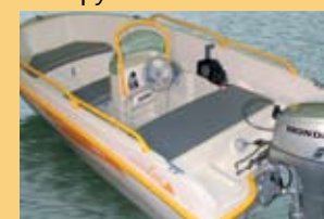
Cushions, steering console, windshield, windshield rail, railings
