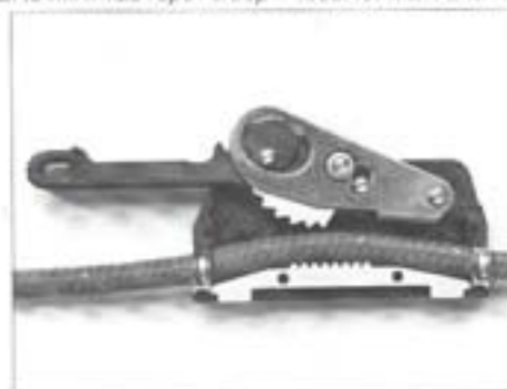
Powerlock operation: Depress lever below horizontal to minimize rope "creep" - ideal for main and genoa halyard control
