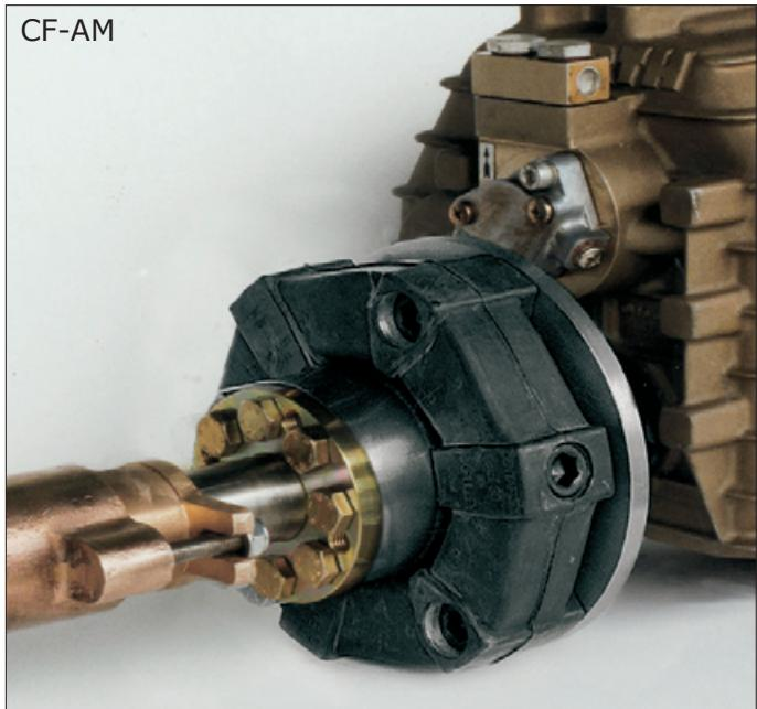
**The CENTAFLEX-M** is available in 2 sizes for 40 and 80 HP approx. depending on propeller shaft speed. Many thousands of these couplings are in service worldwide in motorboats and yachts. Due to the large volume of rubber used, a very smooth transmission of torque and propeller thrust is achieved. The couplings have a fail-safe device which ensures that power can continue to be transmitted even if the rubber fails.
